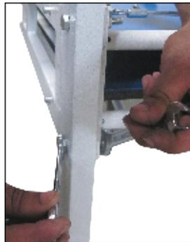
ATTACH WHEEL ASSEMBLY (P4) WITH TABLE FRAME CROSS BAR (P5) USING NUT AND BOLT (P22) AT BOTH SIDES AND TIGHTEN IT WITH THE HELP OF TWO SPANNERS AT BOTH SIDES.
