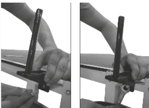
ATTACH POSTS TO THE LEFT AND RIGHT SIDE OF THE TABLE WITH THE HELP OF BOLT (P25) AND TIGHTEN IT WITH THE HELP OF SPANNER (P27).
