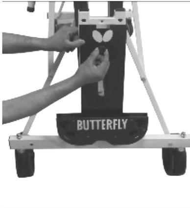
ATTACH BALL AND RACKET HOLDER (P26) WITH WHEEL ASSEMBLY (P4) USING TIGHTENING SCREW (P23) AT BOTH SIDES.
