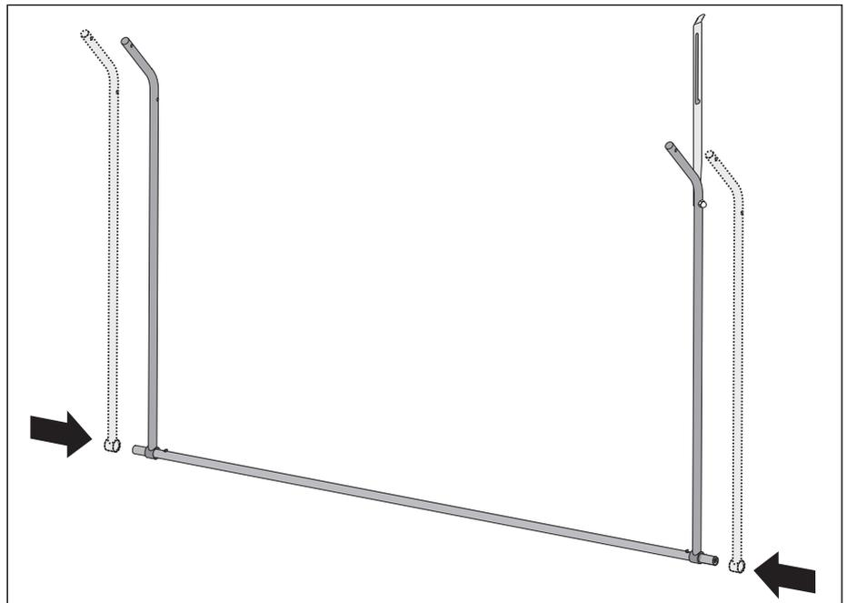
**Attention: By all means, secure the table half against sliding and/or overturning for the subsequent installation steps! First, have a second person bolt the support legs attached to the table with the lateral parts.**
